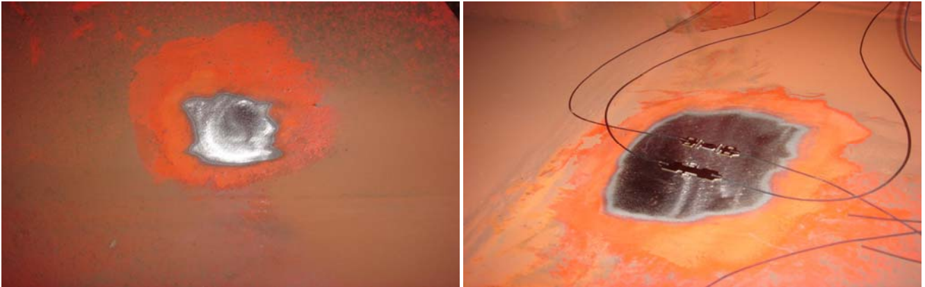
Sensor installation : spot welding
